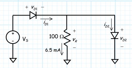
1) If 6.5 mA flows through a 0.1 K resistor, the voltage across that resistor is:
