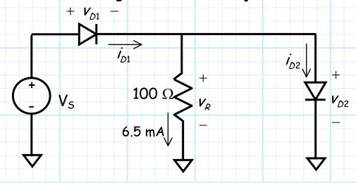
The diodes are identical, with n = 1 and  $I_s = 10^{-14}$  A.
